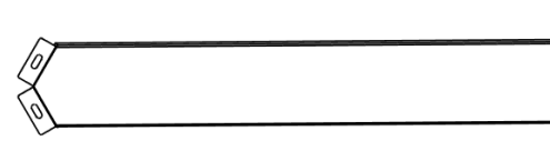
B07 VERTICAL GABLE SUPPORT - A4M04317 (x2) 1 1/2"x9 1/16"x34 11/16" (38x230x882)
