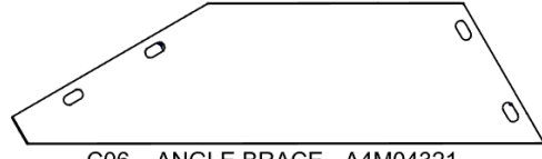
C06 ANGLE BRACE - A4M04321 (x2) 1 7/16"x5 5/16"x20 1/16" (36x135x509)
