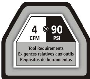
**IMPORTANT:** To operate correctly, this tool requires airflow that is at least 4 cubic feet per minute (CFM) at 90 pounds per square inch (PSI). Check the specifications of your air compressor to be sure that it can support both the minimum CFM and PSI required. An air hose may cause up to 15 PSI drop in pressure, so you may need to set the output higher to maintain the required pressure at the tool.
