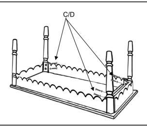
Step 2: Screw the rest 3 legs to the bottom of the bench top using 6pcs screws with washers.
