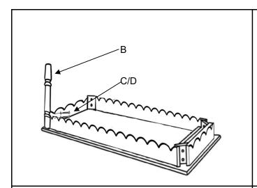
Step 1: Take all packaging off the bench. Screw 1pc leg to the bottom of the bench top using 2pcs screws with washers.
