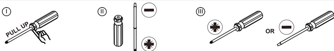
Screwdrivers can be converted to Phillips and Slotted.
