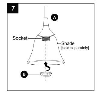
Install one standard-base 60-watt max. incandescent bulb (not included) or CFL/LED equivalent. \*Maximum wattage for fixture (A) is 60 watts--PLEASE NOTE WARNINGS BELOW.
