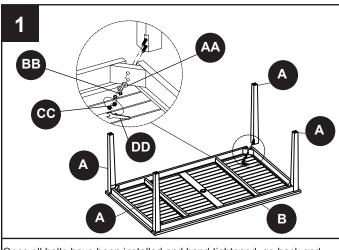
Once all bolts have been installed and hand tightened, go back and tighten firmly with wrench, DD.
