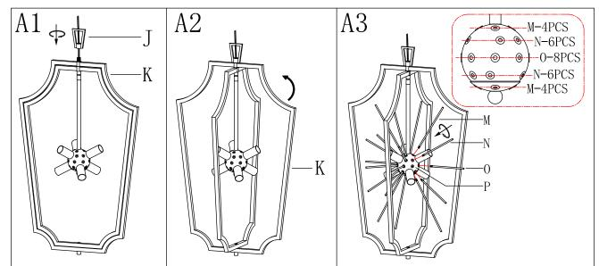
Step A1 » Screw loop (J) onto the top of frames (K).
