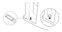
10. Connect the water supply line and turn on the water. Flush several times and check for leaks. Please Do Not Overtighten.
