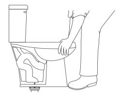
8. Install floor mounting kit as shown below. DO NOT OVERTIGHTEN!
