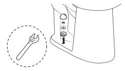
9.Cut excess from the bolt and affix bolt cap
