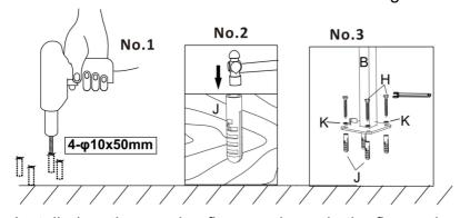
Installed on the wooden floor as shown in the figure above.
