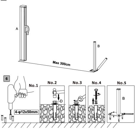
Installed on the concrete floor as shown in the figure above.
