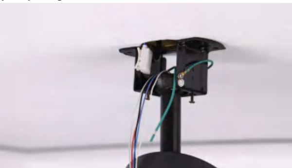
29. Place the downrod ball into the slot in the ceiling bracket. If the slot doesn't align properly then rotate the ball
