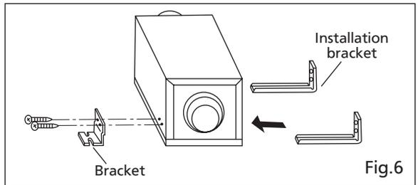
2. Extend installation bracket and put the unit on the ceiling or joist. Secure with long screws. (Fig.7)
