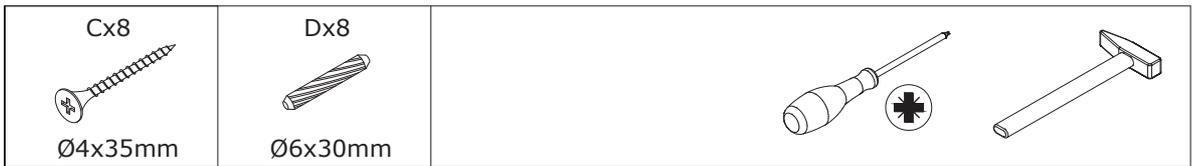
Attach plate 1 to plate 3,5,4 and 2 with wooden dowel(D), then fix using screw(C) as shown.
