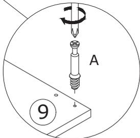
Insert quickfit screw(A) into corresponding holes in plate 8,9 and 11 as shown.
