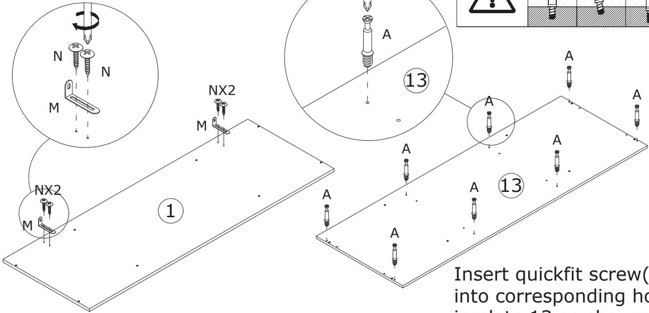
Insert quickfit screw(A) into corresponding holes in plate 13 as shown.
