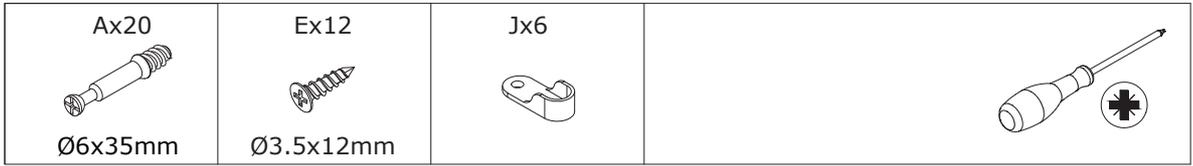
Insert quickfit screw(A) into corresponding holes in plate 2 and 3 with a screwdriver as shown.
