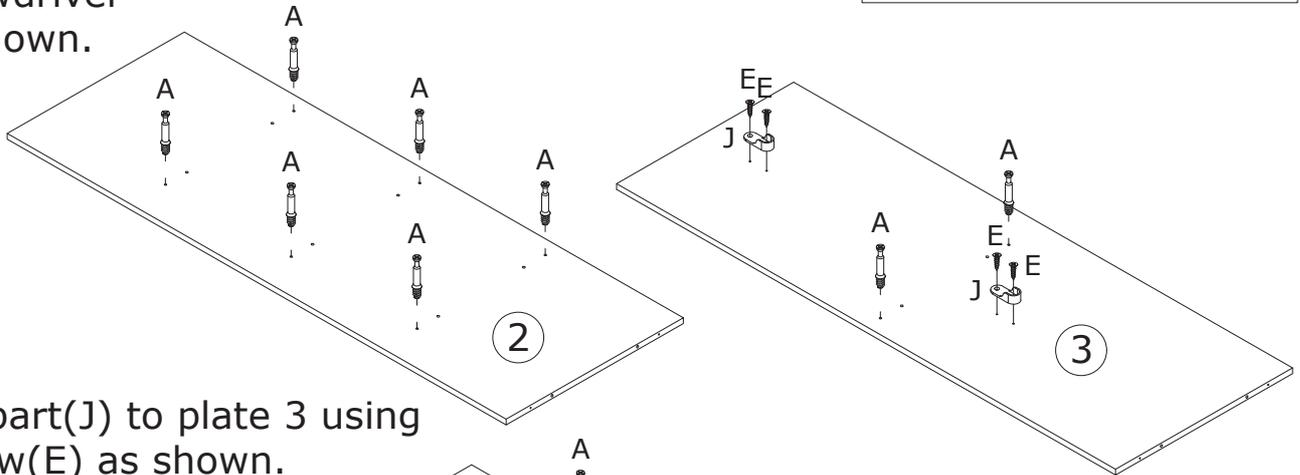
Fix part(J) to plate 3 using screw(E) as shown.
