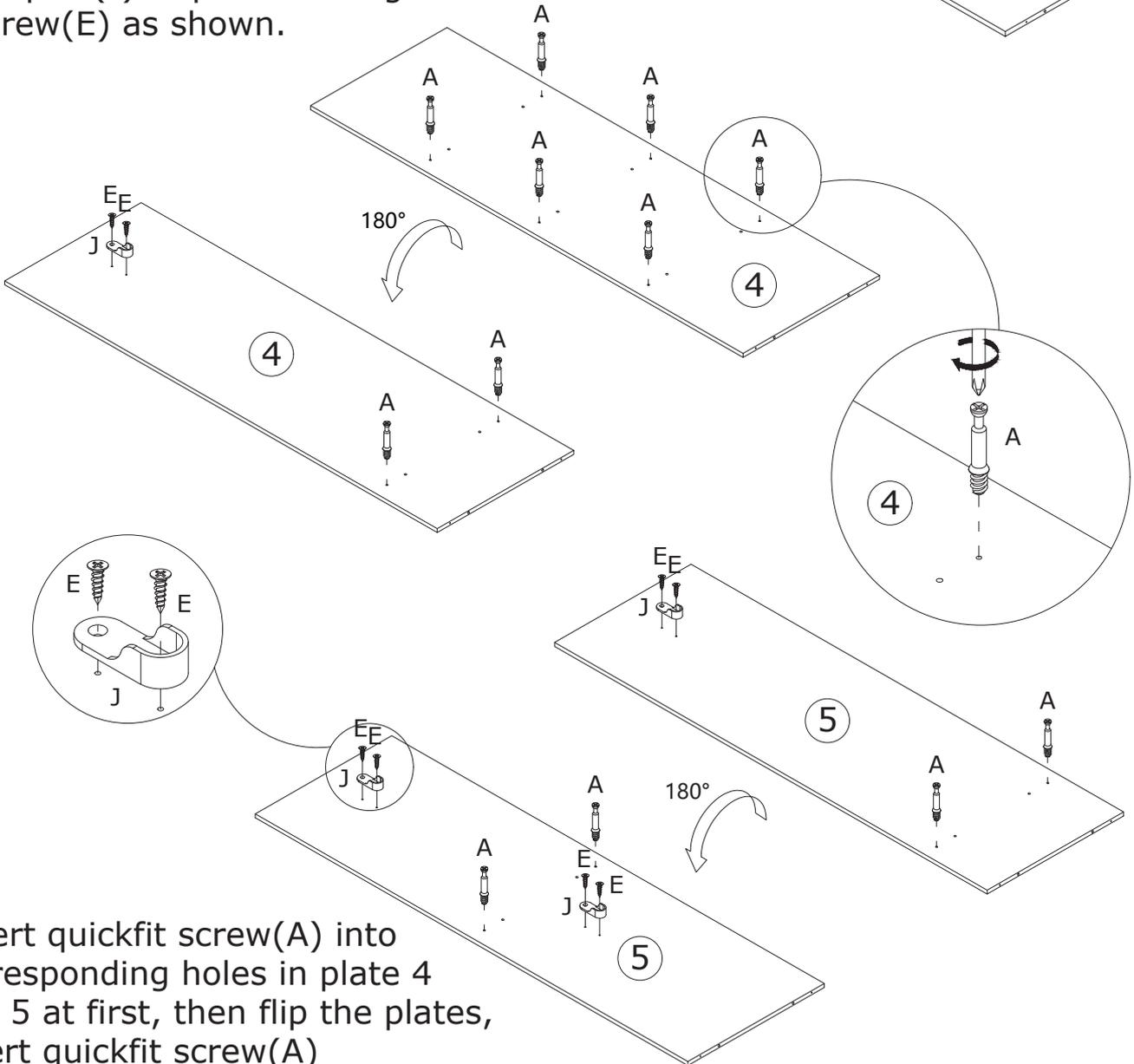
Insert quickfit screw(A) into corresponding holes in plate 4 and 5 at first, then flip the plates, insert quickfit screw(A) and fix part(J) as well.
