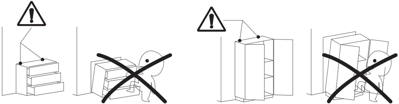
Install anti-tipping device as shown.
