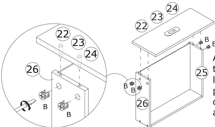
Attach plate 22/23/24 to the drawer, put cam lock(B) into holes in plate 25,26 and turn clockwise to tighten as shown.
