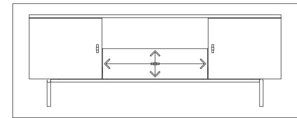
**STEP 15** INSERT THE DRAWER INTO THE UNIT, THEN ADJUST THE DRAWER FRONT PANEL LEFT OR RIGHT AND UP OR DOWN UNTIL THE DRAWER GAPS LOOK PROPORTIONAL.
