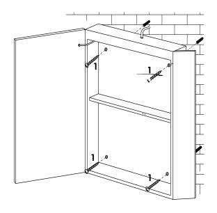
**Note:** When mounting to the wall, the wire can not be pressed between the cabinet and the wall, otherwise the wire installation will be affected.
