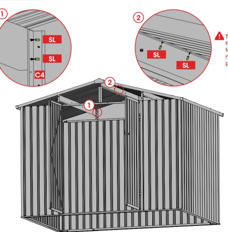
The exposed parts of the upper beam K58-6 and top cover assembly screws need to be covered with plastic protective caps.
