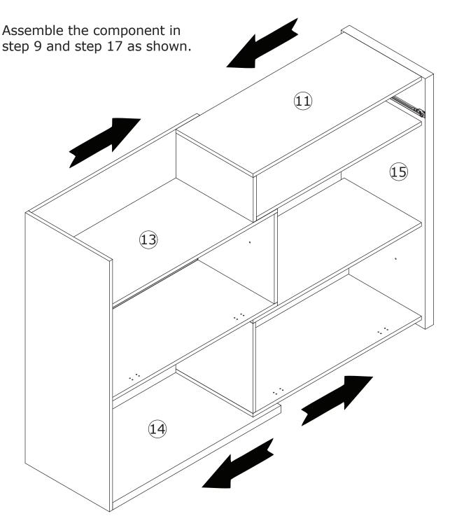
The cabinet can be adjusted left and right according to the space limitation
