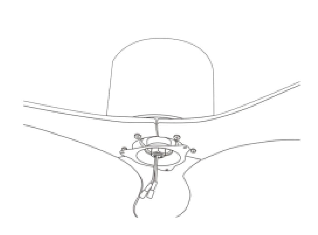
After locking the blade, install the lamp kit
