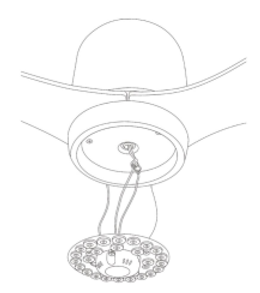
After locking the lamp kit, insert the LED wire ends.
