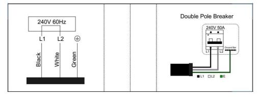
Black live wire L1, white live wire L2, green ground wire. The whole machine cannot be powered on if any of the black and white wires are not contacted well. After the troubleshooting is not a wiring problem: the hob ring does not light up or a single burner does not light up, it may be that the hob is damaged or the power board is damaged.
