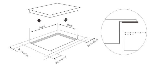
2. It is essential that the Radiant Cooktop is well ventilated and that the air intake and exit are not blocked.
