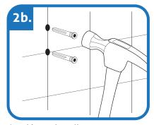
Attaching to drywall: Use drill size appropriate for wall anchors. Tap each anchor in wall with hammer.
