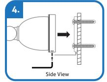
Attach accessory to the mounting plate Use provided hex key to tighten the hex head located on the underside of the accessory to secure the product.
