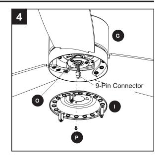
5. Remove one and loosen the other two light pan screws (J) but do not remove from the light pan (I). Connect the 9-pin connector from the light kit (K) and the fitter plate (O). Lift the two keyhole slots in the light kit (K) over the two loosened light pan screws (J). Then, turn the light kit (K) clockwise and re-install the previously removed light pan screw (J). Tighten all three light pan screws (J).
