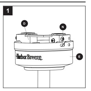
Secure the canopy (E) with the mounting bracket screws (N) previously removed (Step 4, page 8). Tighten all mounting bracket screws (N) securely.
