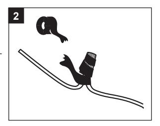
3. Turn the spliced/taped wires upward and gently push the wires and wire connectors (AA) into the outlet box.
