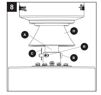
9. Depending on the length of downrod you use, you may need to cut the lead wires back to simplify the wiring. If you decide to cut back the lead wires, take the lead wires and make sure you have pulled them all the way through the top of the downrod. Measure at least 8 inches of lead wire, then cut the excess wire off with wire cutters (not included).
