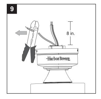
If you decided to cut back the lead wire in Step 9, strip 1/2 in. of insulation from the end of the white wire. Twist the stripped ends of each strand of wire within the insulation with pliers (not included). Repeat this step for black and blue wires.
