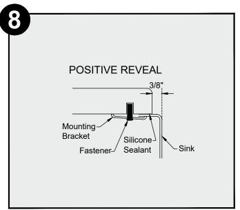
Tighten fasteners to secure the sink. Check the alignment of the sink to the countertop opening. Double check the tightness of the fasteners and remove excess silicone. After silicone has cured, wipe the bead with a wet cloth. This will smooth out any rough areas. Allow sealant to set for 30-60 minutes.
