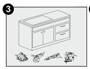
Cut the opening in the countertop by carefully following the traced line. Cut the countertop using the appropriate cutting tools.
