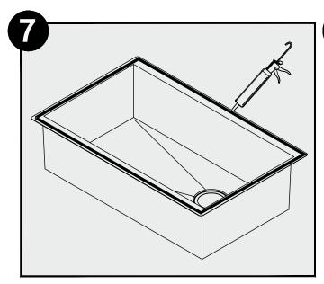
Apply a quality silicone to the underside of the countertop around the perimeter of the sink rim. Position and align the sink in the correct position over the opening and press firmly.
