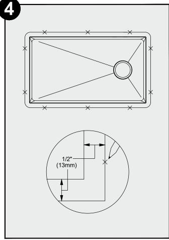
Turn countertop over and align the sink with the countertop. Decide the locations for mounting brackets. Mounting holes should be 1/2" from the edge of the sink.
