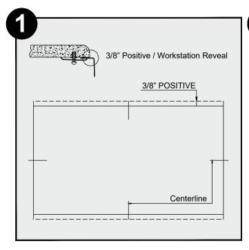
In order to have a workstation ledge, your sink must be installed with a positive reveal. Use scissors to cut along the line of the paper template for your positive reveal.
