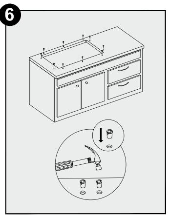
Insert anchors into the drilled holes and lightly tap with a hammer until flush.
