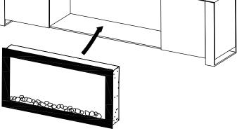
D: Push the fireplace into the mantel , and then fix the fireplace to the mantel with three screws from the back.
