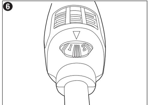
The numbered positions, 1 through 6 inscribed on the variable speed dial, do not indicate any precise speed but are good reference points. The higher the number, the higher the tool speed.
