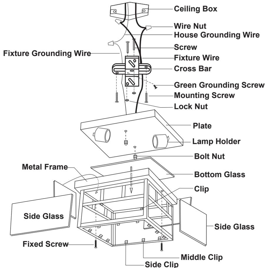
1. Thread two screws through the cross bar, then secure them with two lock nuts. Adjust the length of the screws if necessary.
