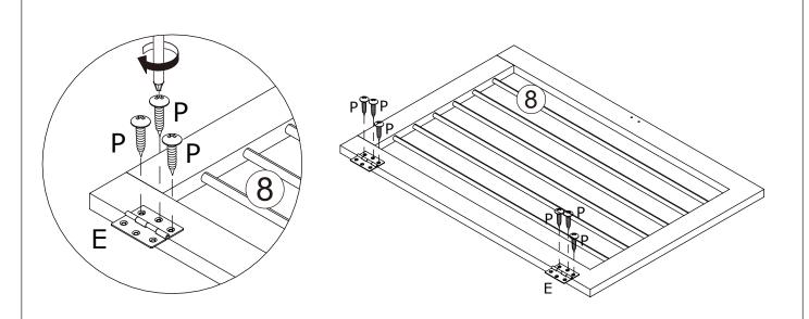
Using screw(P) to lock hinge(E) to panel #8 as shown.
