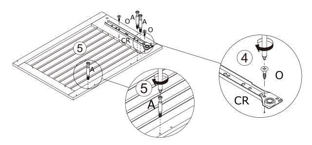
Using screw(O) to connect rail(CR) to panel #5 and insert cam bolt(A) to panel #5 as shown.
