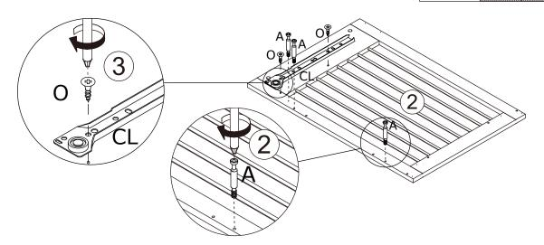
Using screw(O) to connect rail(CL) to panel #2, and insert cam bolt(A) to panel #2 as shown.
