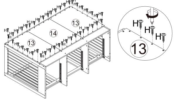
Using screw(H) to fix panel #13,#14 to the cabinet as shown.
