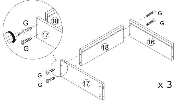
Using screw(G) to fix panel #16,#17 to panel #18 as shown.
