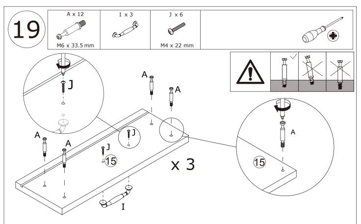
Insert cam bolt(A) to panel #15 as shown.
