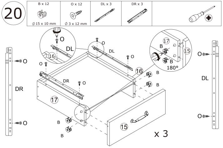
Connect panel #15 with panel #16,#17 and add lock(B) to as shown. Using screw(O) to lock (CL),(CR) to panel #16,#17 as shown.  $^{14/15}$
