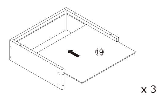
Slide back panel #19 into avaliable slots as shown.
