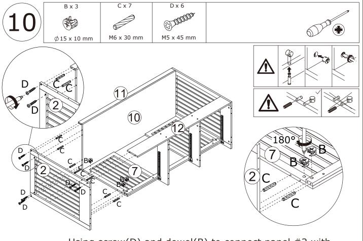
Using screw(D) and dowel(B) to connect panel #2 with panel #7,#10,#11,#12 as shown.
