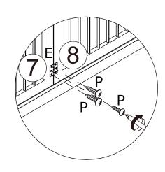
Using screw(O) to connect panel #8 with panel #7 as shown.
