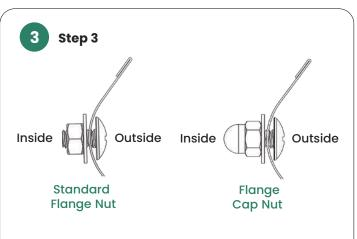
Make sure to tighten each nut and bolt to support the garden raised bed.
