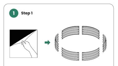
Remove the protective film from all panels, and lay panels on a flat surface to create the round shape.
