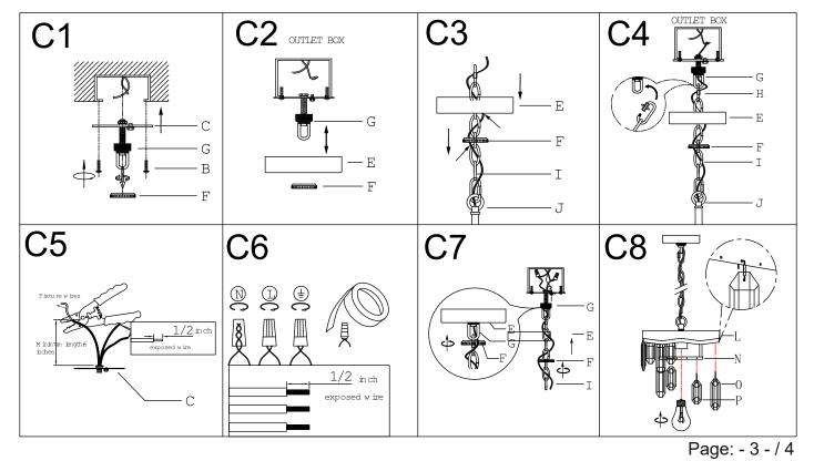
Step C1 » Remove collar ring (F) from collar loop (G). Attach single bar (C) to the outlet box with mounting screws (B).
