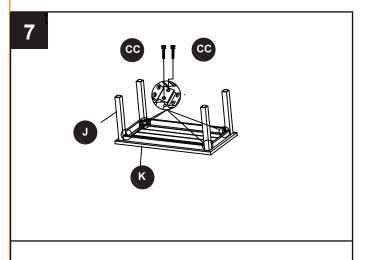
Once all connections are made, tighten CC with EE.
