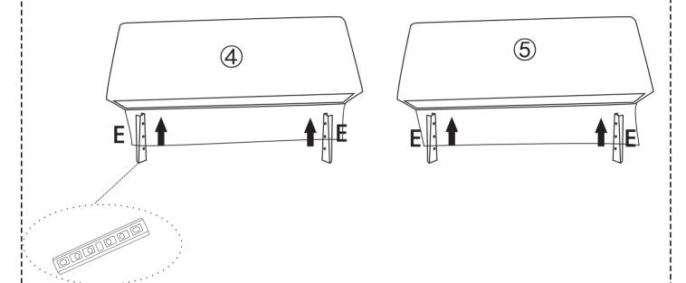
Note: The groove side of the latch is facing outward.
