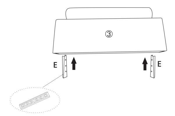
Note: The groove side of the latch is facing outward.
