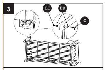
Once all connections are made, hand-tighten DD and EE.
