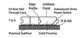
Solid hardwood flooring can be installed on concrete slabs (minimum 3,000 psi) **on or above grade**. The moisture content of the slab should be tested with a Calcium Chloride Test and emit less than 3 pounds per 1,000 square feet per 24 hours, then the appropriate subfloor (nailing surface) can be installed. An installer should record moisture test results in the space provided on page 8 of this document and leave with the owner as part of their records.
