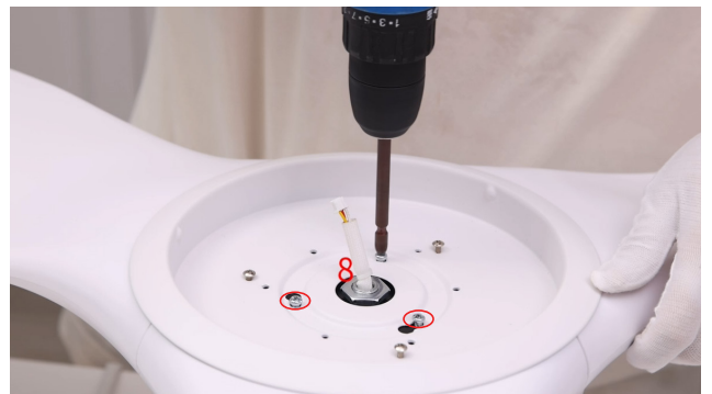
14.Tighten the 3 silver lamp panel screws
