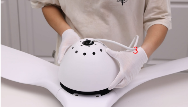
7.Install the motor cover
