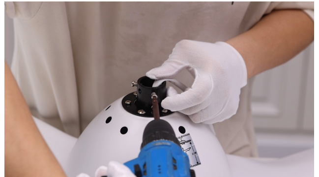
12.Loosen and remove the 3 silver screws pre-locked on the motor (They will be needed later)
