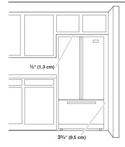
To ensure proper ventilation for your refrigerator, allow for a 1/2" (1.3 cm) space at the top and behind the refrigerator. If your refrigerator has an ice maker, allow extra space at the back for the water line connections. When installing your refrigerator next to a fixed wall, leave 3-3/4" (9.5 cm) minimum space between the refrigerator and wall to allow the door to swing open.
