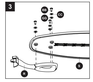
Install the blade arm (R) to the underside of the motor assembly (G) with motor screws (T) previously removed (Step 6, page 8). Tighten with Phillips screwdriver. Repeat for each blade arm (R).
