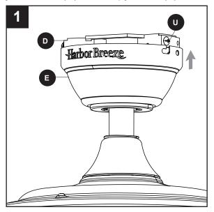
Secure the canopy (E) with the mounting bracket screws (U) previously removed (Step 4, page 8). Tighten all mounting bracket screws (U) securely.
