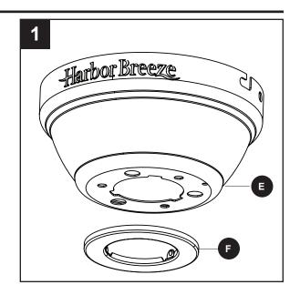
Remove three Phillips-head closemount screws (X) from the top of the motor assembly (G). Align the canopy (E) with the holes in the top of the motor assembly (G), then re-install the Phillips-head closemount screws (X) to secure the canopy (E) to the top of the motor assembly (G).
