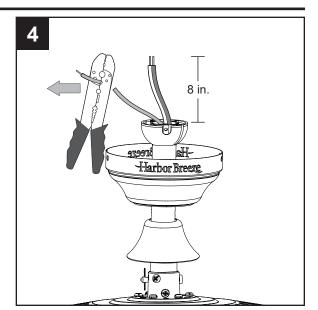
If you decided to cut back the lead wire in Step 4, strip 1/2 in. of insulation from the end of the white wire. Twist the stripped ends of each strand of wire within the insulation with pliers (not included). Repeat this step for black and blue wires.
