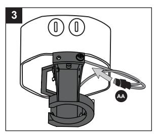
Note: Closemount installation will not have the downrod (A), yoke cover (N) or canopy cover (F).
