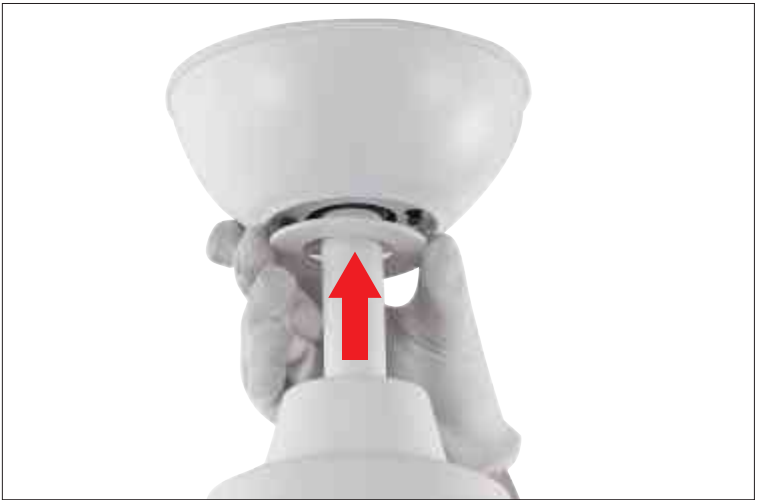
Step 15 Install the canopy cover to the up canopy..
