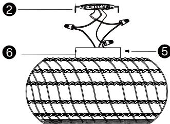
STEP4: Install the Ceiling light fixture onto the mounting plate with two screw B. ( **2** **5** **6** )
