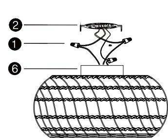
Way 1: Attach the copper wire to ground wire with wire nuts caps. ( **1** )
