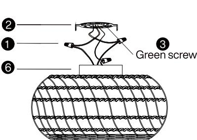
Way 2: Attach copper wire to ground screw(the green screw on the mounting plate)( **1** **2** **3** )
