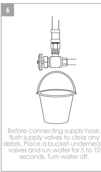
Before connecting supply hose, flush supply valves to clear any debris. Place a bucket underneath valves and run water for 5 to 10 seconds. Turn water off.
