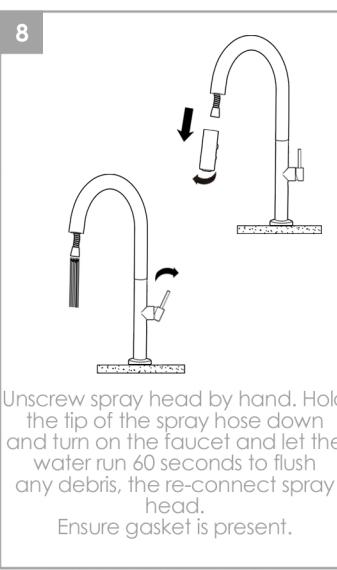
Unscrew spray head by hand. Hold the tip of the spray hose down and turn on the faucet and let the water run 60 seconds to flush any debris, the re-connect spray head. Ensure gasket is present.
