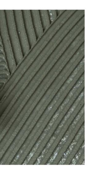
Tile adhesives, traditionally known as cement adhesives, are used to bond tiles to a substrate. They have evolved with the development of new larger tiles with a lower water absorption rate, as is the case of porcelain tiles.
