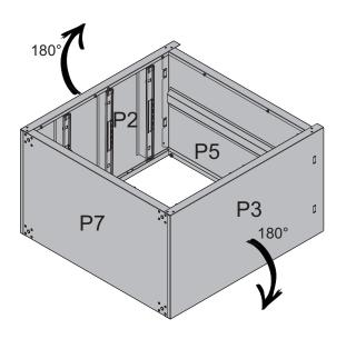
2 - Fit parts **P2** and **P3** to parts **P5** and **P7** with **F1**
