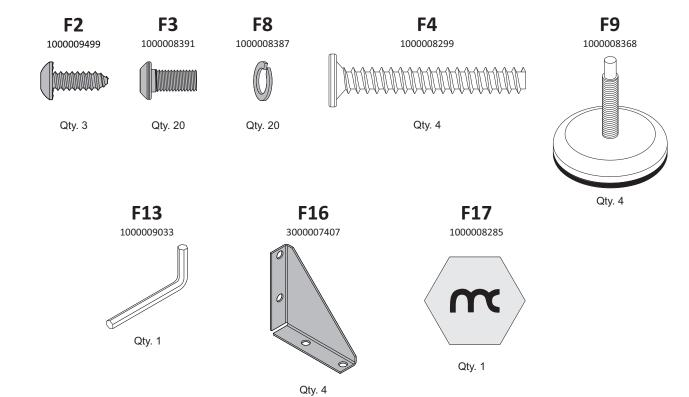
**STEP 1** 1.Fit the shoes to frame **P32** and **P31** base and turn to screw. To level the height or the table, turn the shoe clockwise or counterclockwise until is aligned
