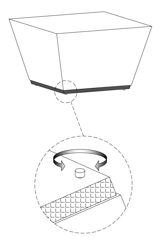
**Note:** Levelers on the bottom can be adjusted if floor is uneven.
