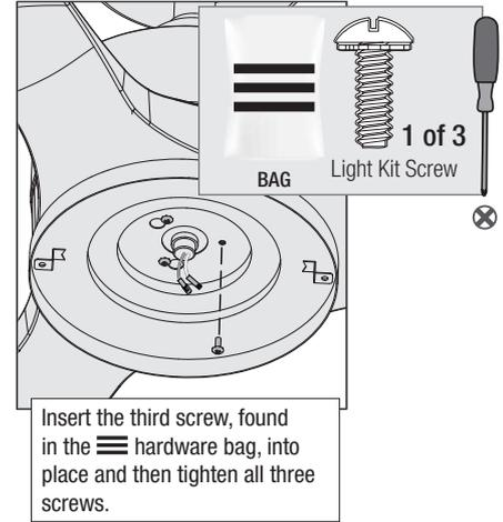
Insert the third screw, found in the hardware bag, into place and then tighten all three screws.
