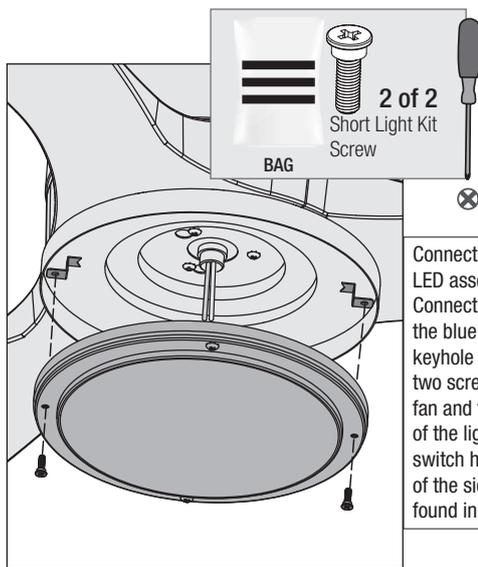
Connect the single-pin connectors from the LED assembly to the connectors from the fan. Connect the white wires together. Connect the blue and black wires together. Align the keyhole slots in the light kit housing with the two screws. Make sure all the wires from the fan and the light kit are snug inside the center of the light kit, not pinched in between the upper switch housing and the light kit or hanging out of the sides. Install two of the light kit screws found in the bag.
