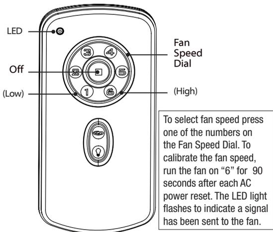
To select fan speed press one of the numbers on the Fan Speed Dial. To calibrate the fan speed, run the fan on "6" for 90 seconds after each AC power reset. The LED light flashes to indicate a signal has been sent to the fan.
