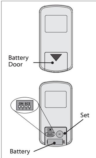
Remove battery door. Change the dip switch settings if they match a previously installed remote transmitter. Install A23 or MN21 alkaline battery in the proper polarity and replace the battery door. To pair the remote, hold down the Set button for 5 seconds. Pairing is complete when LED button flashes twice.
