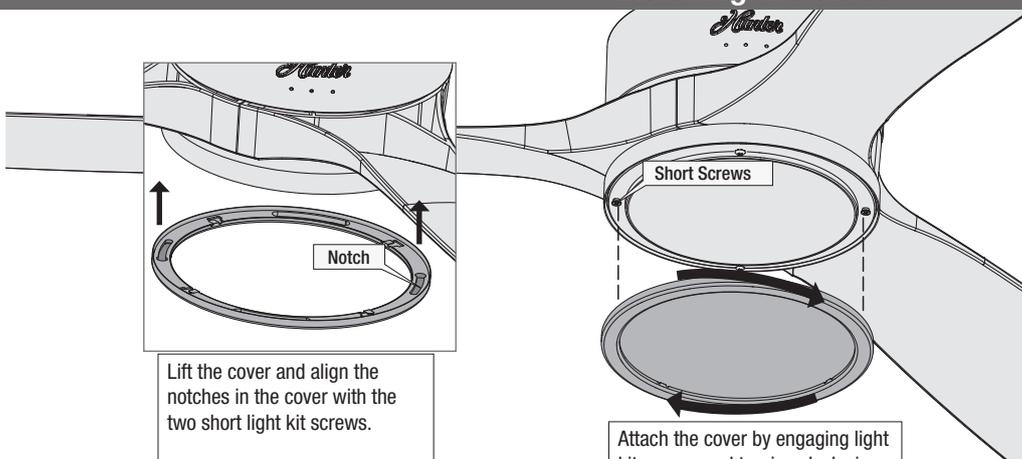
Lift the cover and align the notches in the cover with the two short light kit screws.
