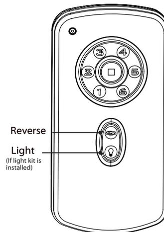
To reverse the air flow direction, press the Reverse button while fan is running. Press Light button to turn lights off/on. To dim the lights, press the light button for more than one second. Light will cycle from brightest to dimmest. Release the light button when desired brightness is achieved.
