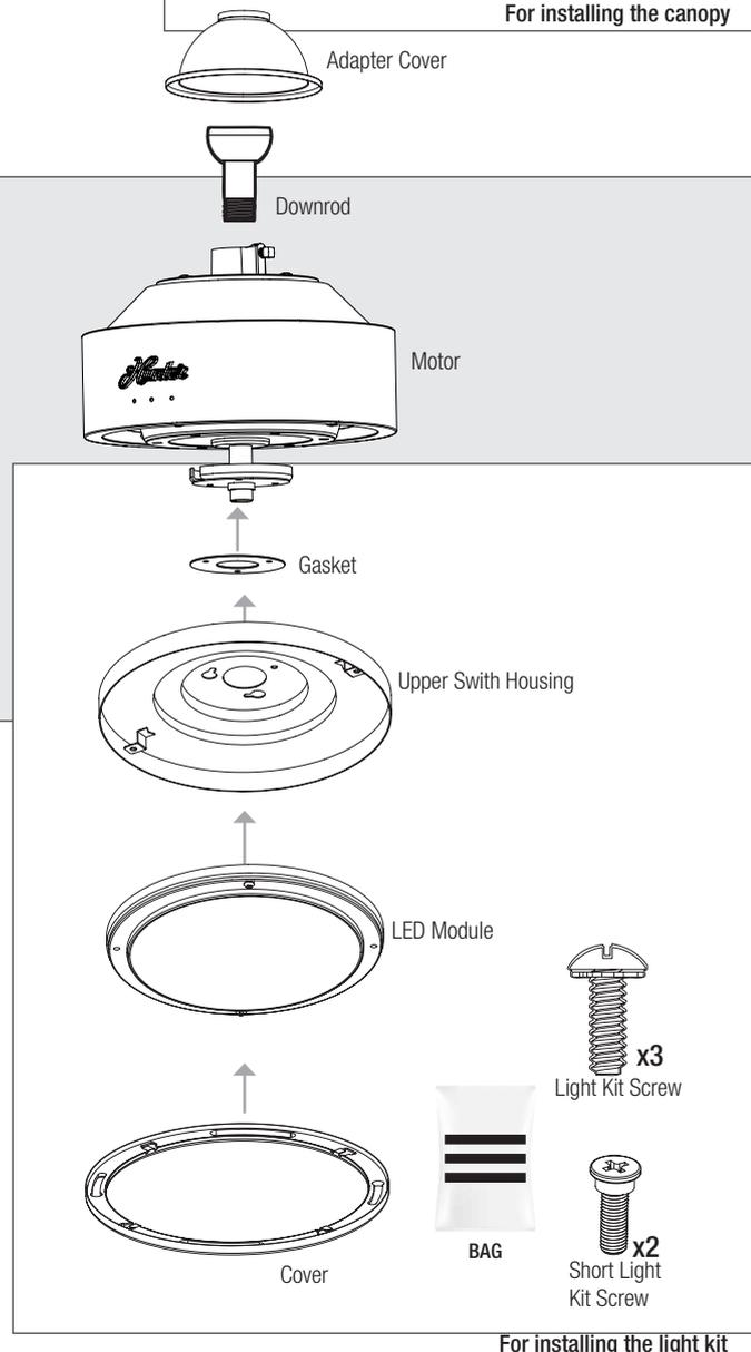
For installing the light kit
