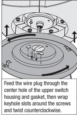
Feed the wire plug through the center hole of the upper switch housing and gasket, then wrap keyhole slots around the screws and twist counterclockwise.
