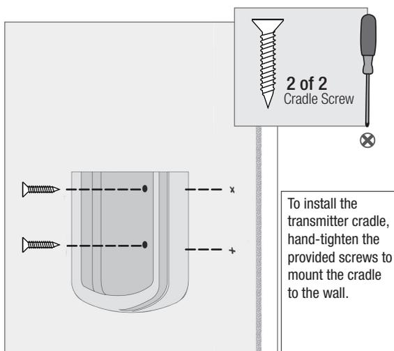
To install the transmitter cradle, hand-tighten the provided screws to mount the cradle to the wall.
