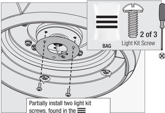
Partially install two light kit screws, found in the hardware bag, through the gasket halfway into the motor housing as shown. It does not matter which two screw holes you choose.
