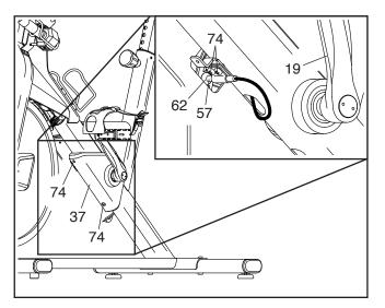
**See the inset drawing.** Locate the Reed Switch (57). Slightly loosen the two indicated M4 x 12mm Blunt Screws (74). Then, turn the Left Crank Arm (19) until a Magnet (62) is aligned with the Reed Switch. Slide the Reed Switch slightly toward or away from the Magnet. Then, retighten the Blunt Screws.
