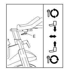
Note: The adjustment handle (E) functions like a ratchet. Turn the adjustment handle in the desired direction, pull it downward, turn it in the opposite direction, push it upward, and then turn it in the desired direction again. Repeat this process as many times as necessary.
