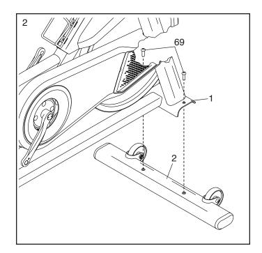
3. Attach the Rear Stabilizer (3) to the Frame (1) with two M8 x 25mm Screws (69).
