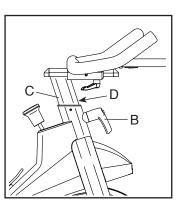
dlebar post, and tighten the adjustment knob four turns. **Make sure that the adjustment knob is engaged in an adjustment hole.** Then, pull the adjustment knob outward, turn it so that it points downward as shown, and then release it.
