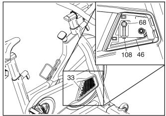
**See the inset drawing.** Loosen, but do not remove, the M8 Jam Locknut (68). Then, tighten the Idler Screw (108) until the Drive Belt (46) is tight. Then, firmly tighten the Jam Locknut.
