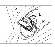
adjust the toe straps to the desired position, and then release the tabs.
