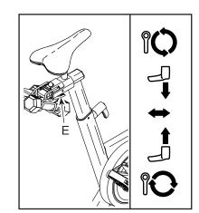
Note: The adjustment handle (E) functions like a ratchet. Turn the adjustment handle in the desired direction, pull it downward, turn it in the opposite direction, push it upward, and then turn it in the desired direction again. Repeat this process as many times as necessary.
