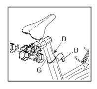
into one of the adjustment holes (D) in the seat post, and tighten the adjustment knob. **Make sure that the adjustment knob is engaged in an adjustment hole.** Then, pull the adjustment knob outward, turn it so that it points downward as shown, and then release it.
