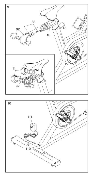
10. Plug the Power Adapter (111) into the Receptacle (110) on the rear of the exercise bike.
