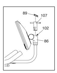
If the console does not stay in place when it is tilted upward and downward, first tilt the console upward as far as possible. Then, use the included small hex key (B) to slightly tighten the two M6 x 16mm Cap Screws (105) inside of the Console Head (86).
