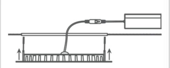
3. Holding the clips place the fixture into the installation hole
