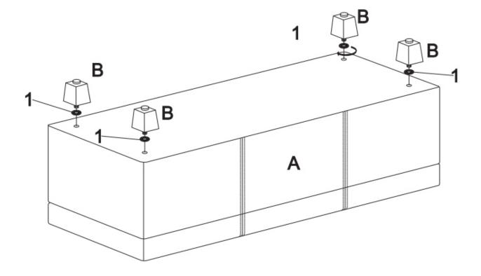
Place the Ottoman (A) on its back on a flat smooth surface. Attach the Feet (B) with Washer (1) to each corner. STEP 2
