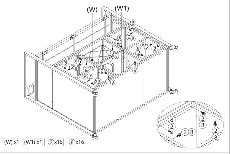
**Step 14:** Connect Door Frame (T) (on the left) with (W), door frame (U) with (W1) (on the right) with bolt (4)-no use washer (8).
