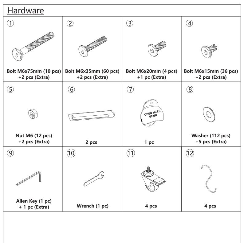
**Step 1:** Connect the wheel sets (11) (in the hardware) to the left frame (A) and right frame (B). Insert frame (C) into the left frame (A) and right frame (B).
