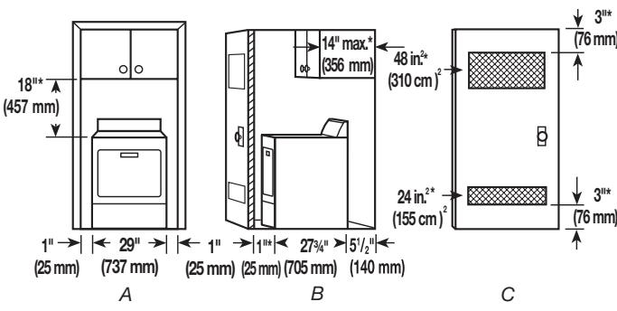
For closet installation, with a door, the minimum ventilation openings in the top and bottom of the door are required. Louvered doors with equivalent air ventilation openings are acceptable.
