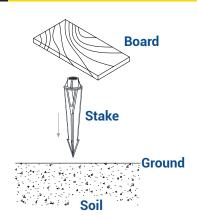
Determine your desired location for mounting the transformer. Hammer the stake into the ground until flange of stake is flush to grade. To avoid damage to the stake, place a board on top of the stake while hammering.
