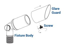
Loosen the screw and remove the glare guard from the fixture body.
