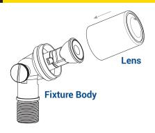
Screw the lens top back onto the fixture body and hand tighten until snug.
