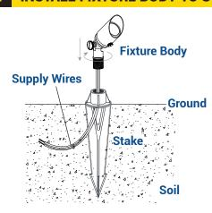
Pass supply wires through the center of the stake and thread the fixture body onto the stake. Hand tighten until snug. Clear away area in ground and lay supply wires into wireway slots.
