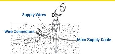
Strip two leads from fixture supply wires. Using two UL listed wire connectors (not provided), connect leads from fixture supply wires to main supply cable leads.
