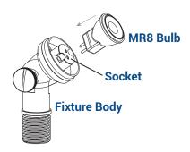
Insert MR8 bulb with correct wattage and type marked on fixture label.
