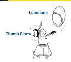
Loosen the thumb screw at the joint and adjust the luminaire to your desired direction. Always tighten the thumb screw after adjustment.
