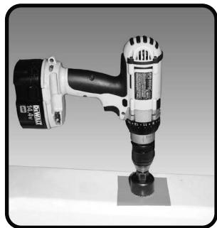
Step 3 - Using a 1/2" diamond tip hole saw, proceed to drill the large hole. Keep drill speed on the slowest speed and use lubricating oil or liquid soap to keep the hole saw cool during cutting.
