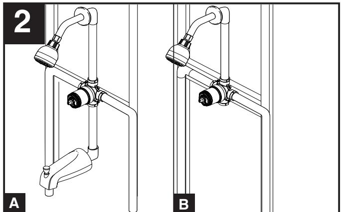
Connect water supplies to left (hot) and right (cold) valve body inlets using proper fittings for your valve body type (iron pipe, copper tubing or pex). Iron pipe connections are shown. Note: For PEX, be sure to use the right fitting and tool for crimping. Connect top outlet (1) to shower arm (2). Insert wall end of shower arm into flange (3) before screwing arm into riser connection (4). Do not use PEX tubing for tub spout drop.
