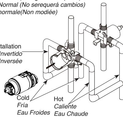
For back to back or reverse installations (hot on right and cold on left) insert the cartridge with the "hot side" on the right. If you are not making a reverse or back to back installation skip this step and continue with step 3.
