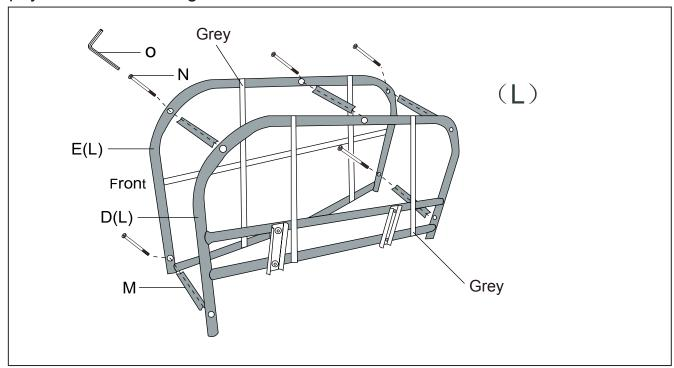
**STEP 2:**Align the armrest cover to armrest-assembled iron frame in sequence <sup>r</sup>ofleft and right, back and forward. so that the cloth cover hole is aligned with the insert hole. Pull the zipper after all is OK.
