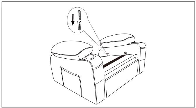
**STEP 7:**Connect the hand controller (Y), then connect the power adapter (I) to the motor cable, and lock locking cables, finally, connect the power cord (X) to the power adapter (I), spread out the leg rest using the controller.
